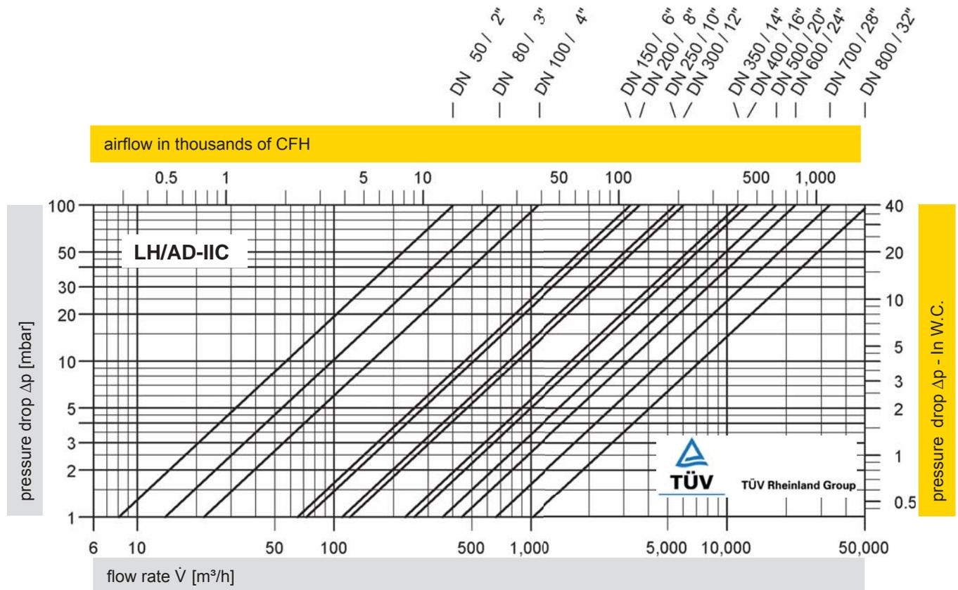
The flow capacity charts have been determined with a calibrated and TÜV certified flow capacity test rig.
