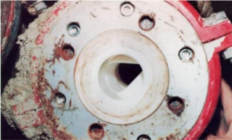
Ceramic ball and body of rotary control valve are still in like-new condition after months of service with extremely erosive slurry
